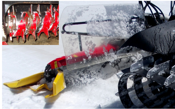
FIGURE 4.4 – The tiller is mounted at the rear of a grooming machine and consists of a high speed rotating shaft (cutter bar) with multiple tines which acts as a mixer for the top of the snowpack
