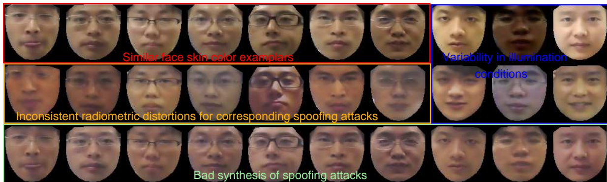
Figure 4.19: Results of the synthesis of print attacks corresponding to low quality acquisitions from the CASIA database. First row corresponds to enrolled face from the testing set. Second row corresponds to spoofing attacks ground truth. Third row displays synthesized fake faces using the proposed method.
