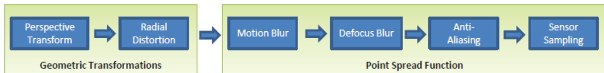
Figure 4.3: Image formation from an optical perspective
