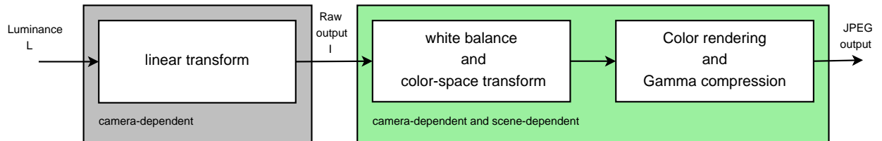
Figure 4.2: Image formation from radiometric perspective.
