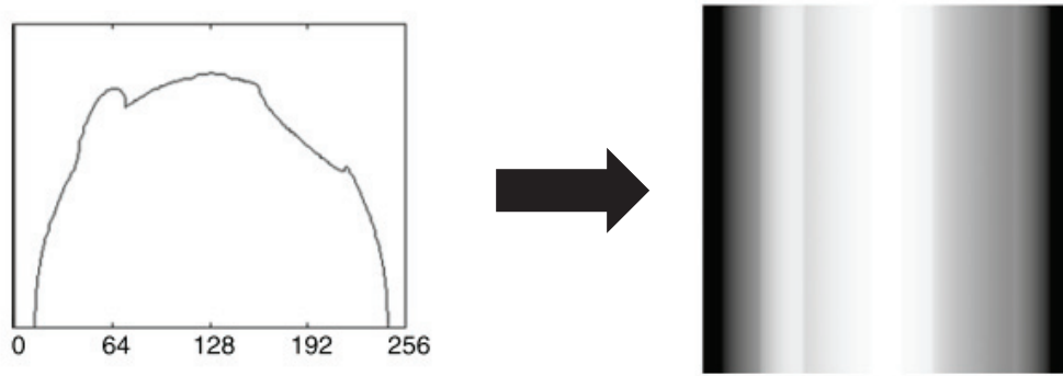
Figure 15 Illustration of the backprojection of one single projection: projection for angle \theta = 0 and its backprojection (Peyrin and Engelke, 2012)
