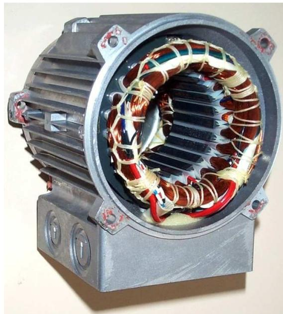
Figure 1 *Stator de machine asynchrone*
