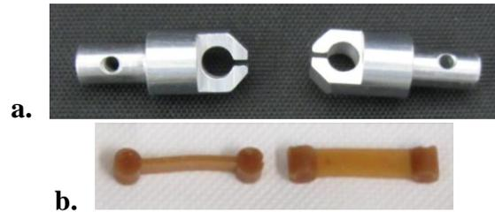
Figure 2. Clamps (a) and samples (b) for in situ X-ray scattering tensile experiments.
