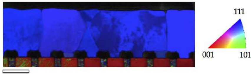
Figure 80: ACOM mapping of the cross-section of an as-is module, showing a strong \langle 111 \rangle texture of the Al grains along the deposition direction. The standard stereographic triangle gives the color codes of the grain orientations, taken here along the vertical growth direction. Scale bar 2.5 \mu\text{m} .
