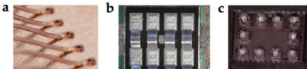
Figure 14: Examples of internal bonding connections in a low voltage power module. (a) Cu bonding wires, (b) Al ribbons, (c) ball-bonding [San17].
