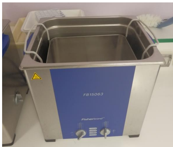
Figure 4.2: Homogenizing process by using a mortar and a pestle as well as an ultrasonic bath.
