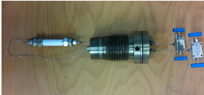
Figure 4-6 Connections between the reaction cell and the capillary tubings and between the capillary tubings and the vessel head.
