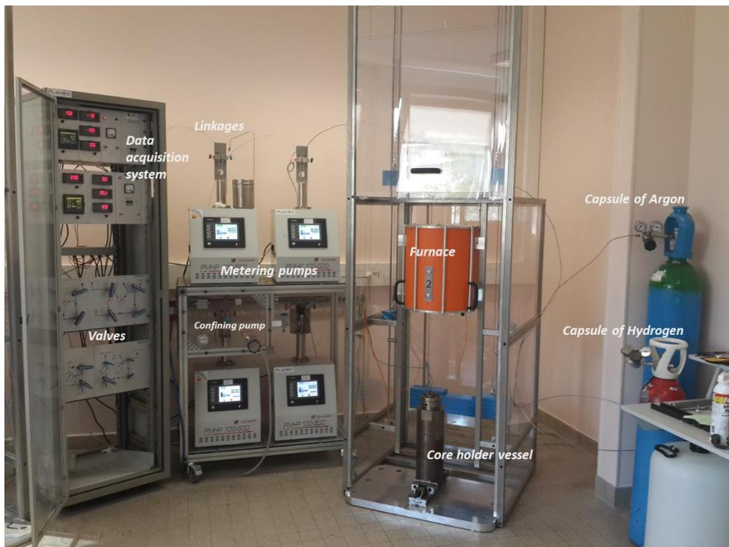
Figure 4-1 General view of the core-flooding experimental set-up.
