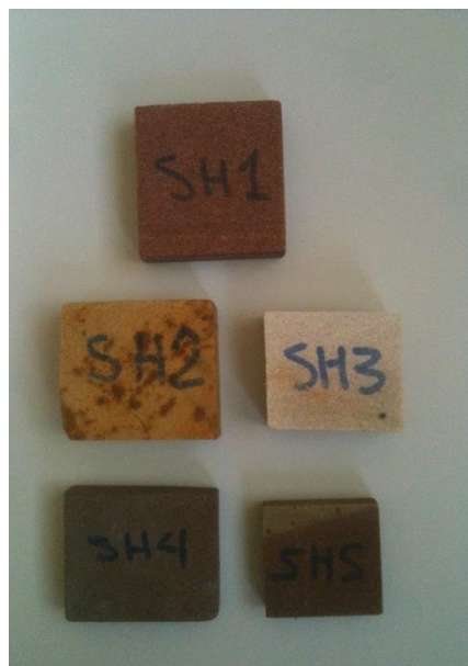
Figure 3-2 Adamswiller, Cleebourg and Rotbach sandstone rock samples
