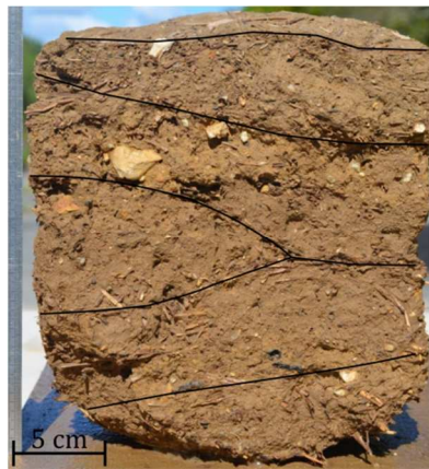
Figure 42. Cob clods limits of a wall portion underlined on a picture (on left) and depicted on a 3-dimension schematic diagram (on right, dimensions in cm).
