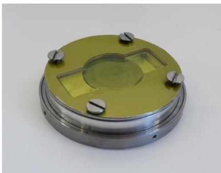
Figure A.1 : Air-tight XRD sample holder used for air sensitive samples.
