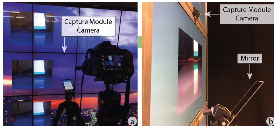
Figure 44: Setup for CamRay 's performance tests. (a) A timer was recorded by one of the Capture Module cameras mounted on WILDER and looped back to the display for the local performance test. Both the timer and its video are recorded by a video camera. (b) For the remote performance test, a mirror reflected the video of the timer in WILDER , which was recorded by a Capture Module in this room and sent back to WILDER for the remote performance test.
