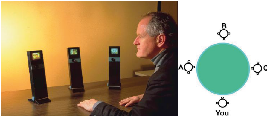
Figure 4: Sellen et al.'s [92] Hydras conferencing system, a remote conferencing system that preserves gaze direction to remote partners by placing their video feeds in a way that reflects their original position. Image from [21].
