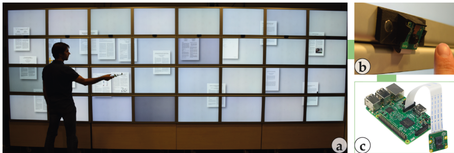
Figure 42: The CamRay Hardware in the WILD wall-sized display. (a) The WILD wall-sized display with one camera in each column on the top row of monitors. (b) A closeup of the Camera Module for Raspberry Pi . (c) The Raspberry Pi computer at the back of a monitor with its camera attached.
