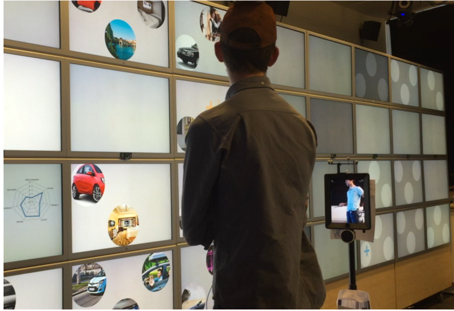
Figure 57: A user in front of a wall-sized display collaborating with a remote person through a telepresence robot.
