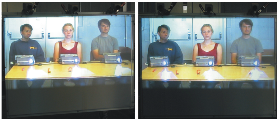
Figure 5: Nguyen et al.'s Multiview conferencing system. Each participant sees the remote participants' gaze direction as in a face-to-face situation. Image from [82].
