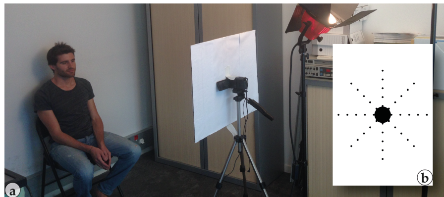
Figure 28: Video recording setup. (a) A camera records an actor gazing at the targets (b), printed and placed in front of him. The camera is placed at the center of the targets.
