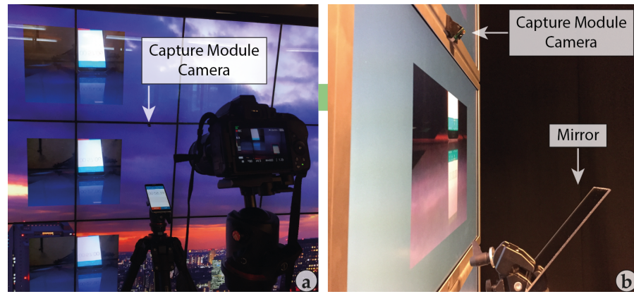
Figure 44: Setup for CamRay 's performance tests. (a) A timer was recorded by one of the Capture Module cameras mounted on WILDER and looped back to the display for the local performance test. Both the timer and its video are recorded by a video camera. (b) For the remote performance test, a mirror reflected the video of the timer in WILD , which was recorded by a Capture Module in this room and sent back to WILDER for the remote performance test.
