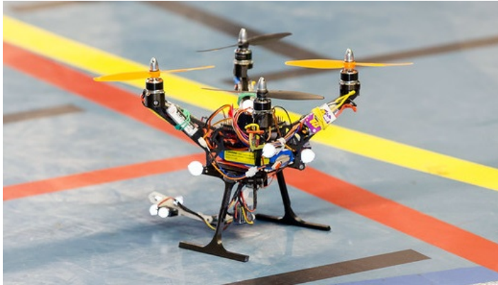
Figure 5.5 – The mini-quadcopter with its arm manipulator.
