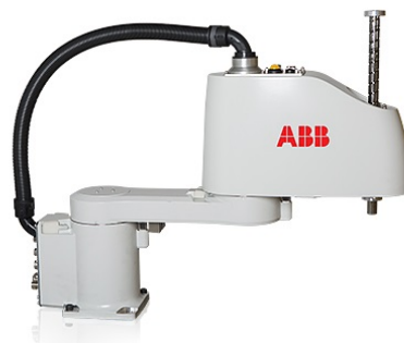
Figure 1.7 – Type I SCARA configuration, courtesy of (ABB [2016]).
