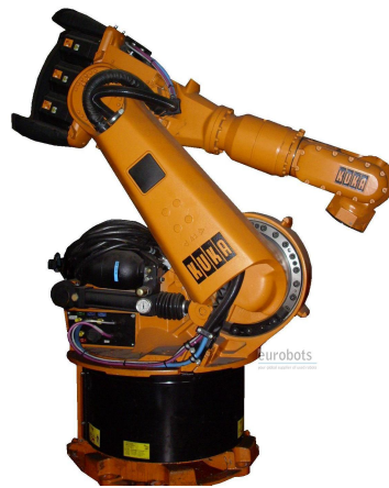
Figure 1.6 – Articulated robot arm configuration, courtesy of (KUKA [2016]).
