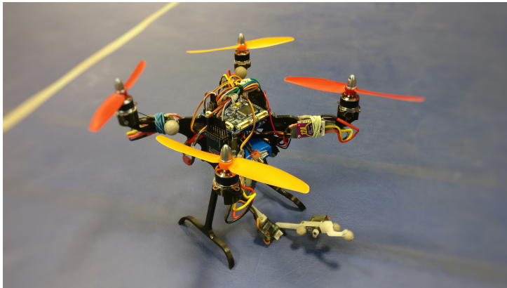
Figure 2.12 – Mini-quadcopter with its manipulator arm.
