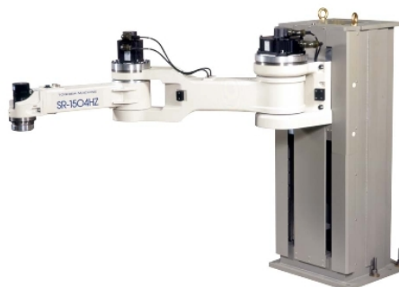
Figure 1.8 – Type II SCARA configuration, courtesy of (Toshiba [2016]).
