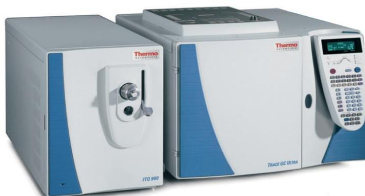
Figure 22 : TRACE GC Ultra- DSQ II MS Thermo Fisher Scientific
