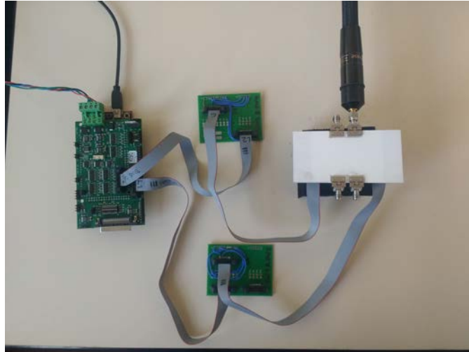
Figure 5.27: Setup for the measurement of the input reflection coefficient.
