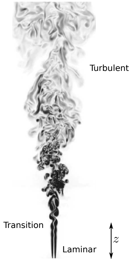
Figure 1.4: Illustration of a laminar to turbulent transition in a buoyant jet flow, M. Masoudian personal contribution, DNS of a turbulent jet [Mas].
