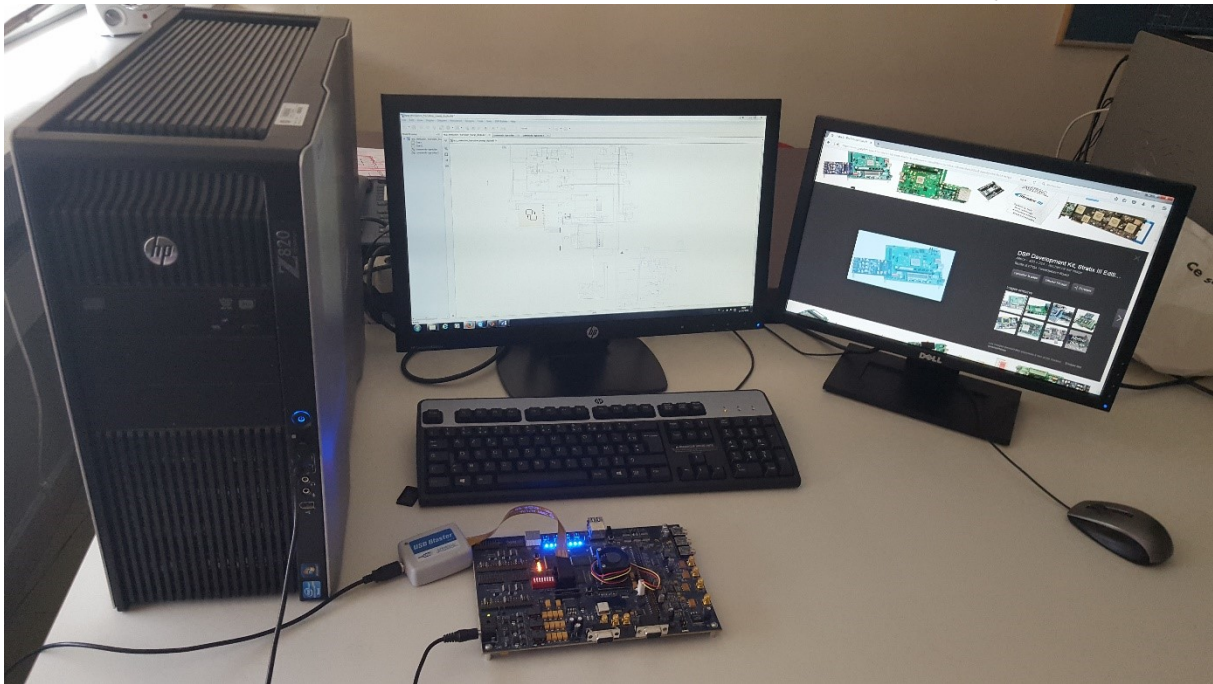
Figure V. 3 : Principe du prototypage “FPGA in the loop”.
