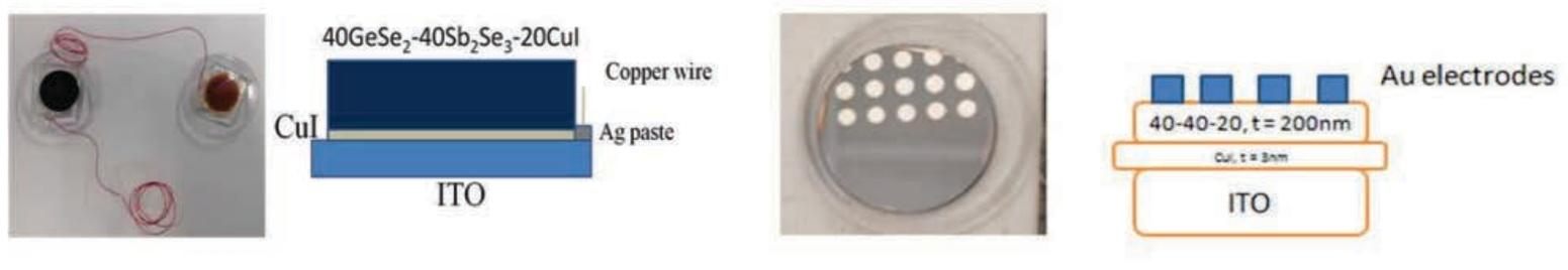
Figure 4-27 Samples for PEC (left) and PV (right) measurements
