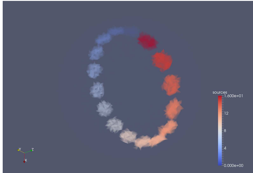
Figure 5.4.7: This figure shows the 3d volume isometric representation of elements selected to be the N_s sources seen in fig. 5.4.5 the diffusion problem.
