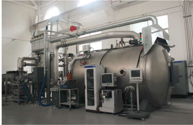
Figure 2.3 The MultiCoat™ hybrid plasma-coating system at GINM [5].
