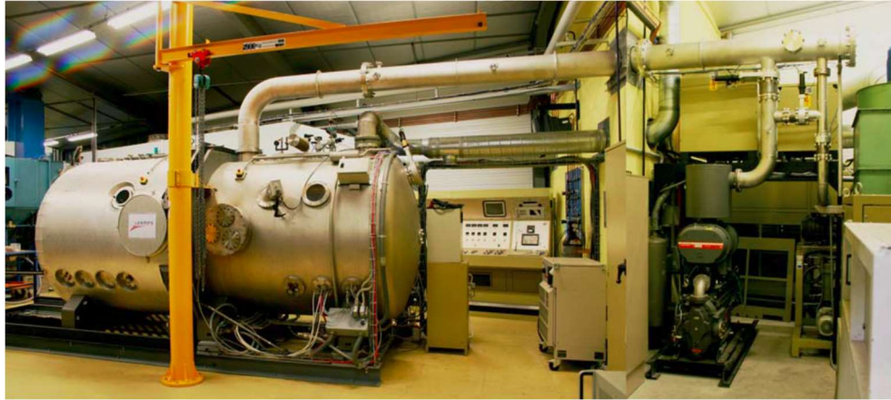
Figure 2.1 The LPPS system made by the LERMPS [3].
