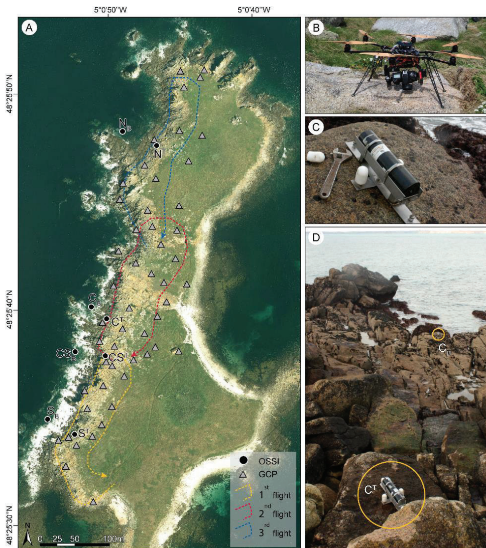
Figure 2-4. Instrumental deployment on Banneg Island. Map (A) shows the drone flight tracks and the location of the ground control points and pressure sensors. Photographs (B–C–D) show the unnamed aerial system, the stainless steel holder for the pressure sensors and the positioning of the sensors along profile C.
