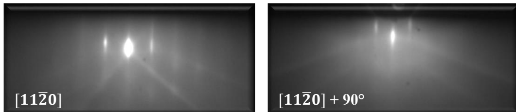
Figure 16. RHEED patterns collected for LNO 128 Y-cut at 500 °C along two azimuths rotated by 90^\circ .
