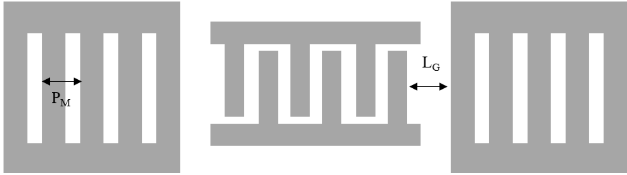
Figure 65. Resonator structure with its characteristic lengths.
