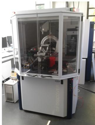
Figure.A. II-2 Photography of the diffractometer used for XRPD in this work
