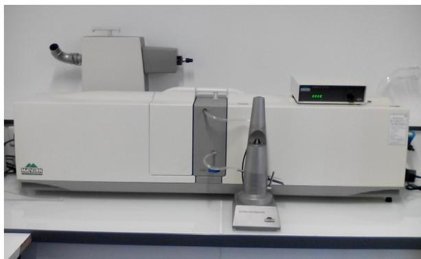
Figure.A. II-7 Photography of the particle size analyzer Mastersizer 2000®
