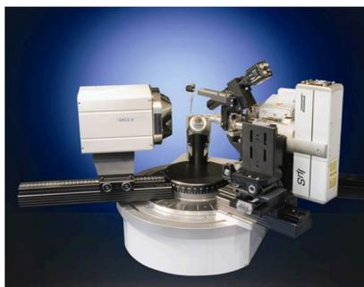
Figure.A. II-1 Photography of the typical device used for SC-XRD in this work.
