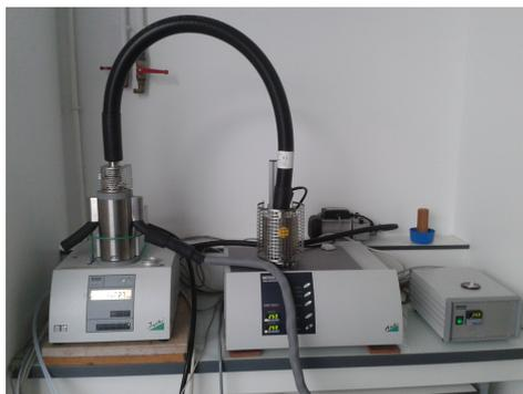
Figure.A. II-4 Photography of the TGA-DSC apparatus used in this work for subambient measurements.
