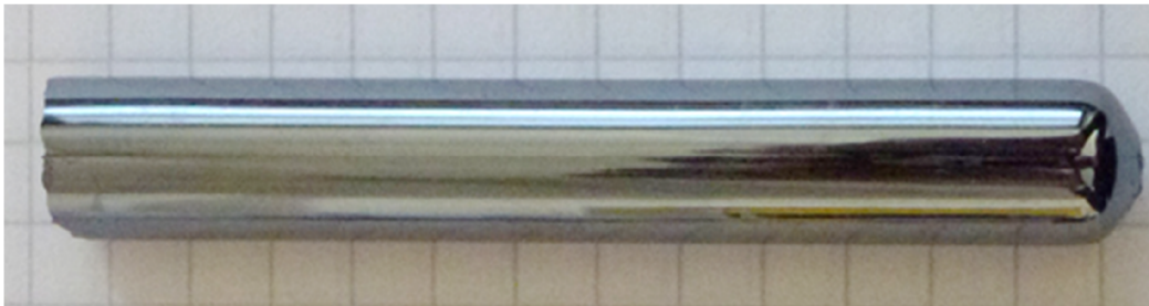
Figure 2.5: Photograph of the glass rod of (GeSe_2)_{90}(Sb_2Se_3)_{10}(2S1G - Se - 3) (diameter 12 mm and length 6.5 cm). Photo taken from Ref. [166].
