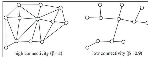
Fig. 2. Two graph models of a road network
