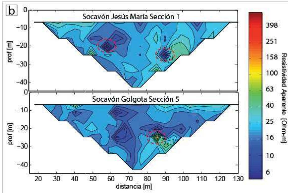
Figure 23 : Pseudo-sections of apparent resistivity. The red dotted lines show the gallery. (a) Two tunnels are observed as conductive areas (<6 Ohm-m). (b) The tunnel is identified as a resistive area (~250 Ohm-m).
