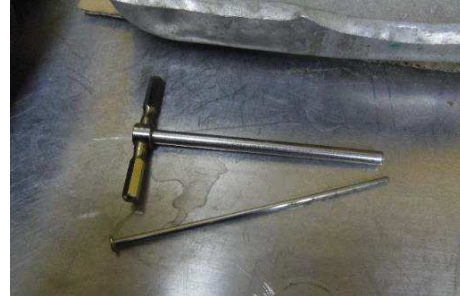
Figure 60 – Equipment used to make the holes for the tensiometers.
