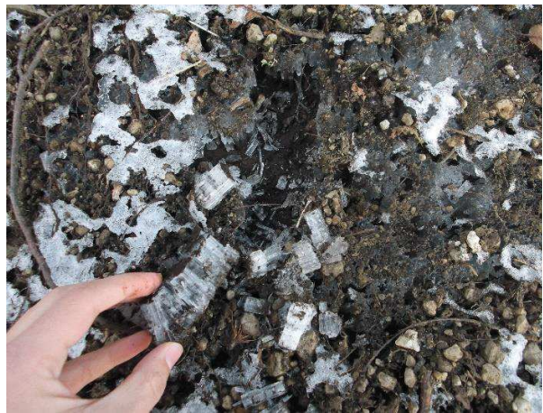
Figure 42 – Formation of a frozen soil layer.
