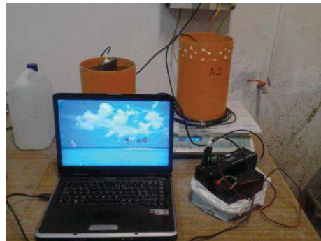
Figure 106 – Equipment used to read the dielectric constant (computer, battery, TDR100 and cables).
