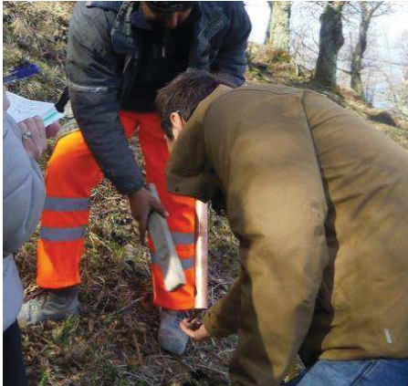
Figure 96 – The soil is being removed from the tube and identified with the help of a geologist.
