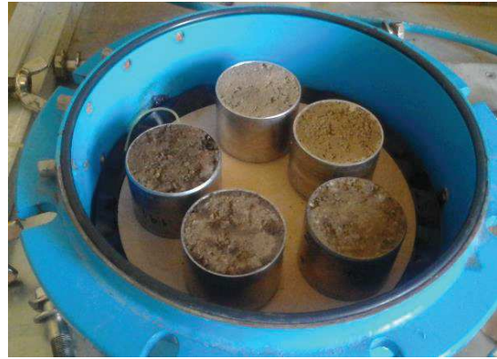
Figure 62 – Position of the samples inside the pressure plate chamber.
