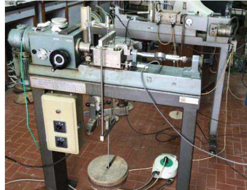
Figure 173 – Traditional direct shear test equipment (Esposito, 2017).
