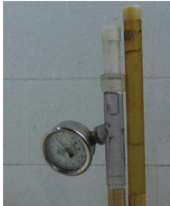
Figure 100 – Vacuum dial gauge and digital measurement adaptor installed on a Jet Fill tensiometer sided with a tradition SDEC France tensiometer.
