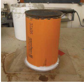
Figure 102 – Plexiglas base glued to the mould.
