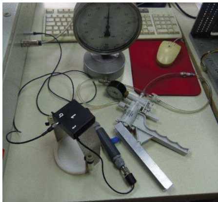
Figure 57 – Setup for the calibration of the tensiometers.
