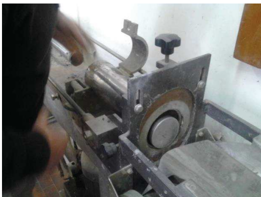
Figure 47 – Soil sample extrusion from the borehole.
