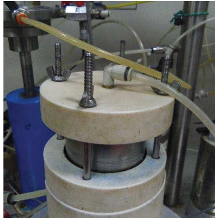
Figure 51 – Permeameter: soil mould and upper and bottom supports.
