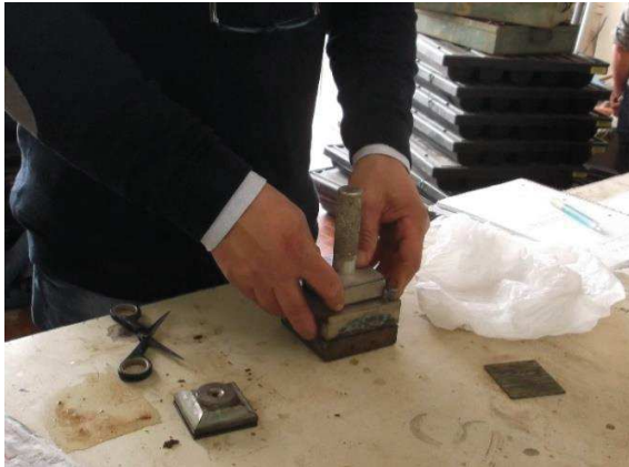
Figure 172 – Insert soil sample in the shear box.
