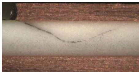
Figure 1.20 – Cracks in Direct Bonded Copper (DBC) [44]
