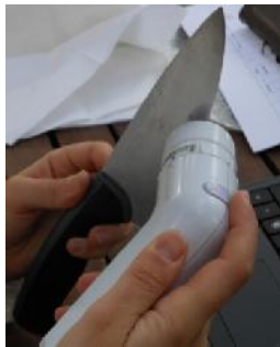
T1 capture images microscopiques lame inox
