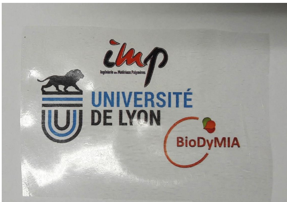
Figure IV-3 : Picture of edible sheet based on casein and 13.2% glycerol (without wax and without KS). Color parameter values are: a^* = -1.60 \pm 0.05 ; b^* = -1.34 \pm 0.02 ; L^* = 40.68 \pm 0.54 .
