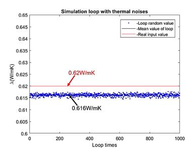
Fig.3-36. Thermal conductivity prediction with less temperature sensors (Annex D)
