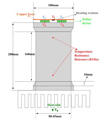
Fig.4-21. Power loss measurement based on calorimetric method with duralumin column
