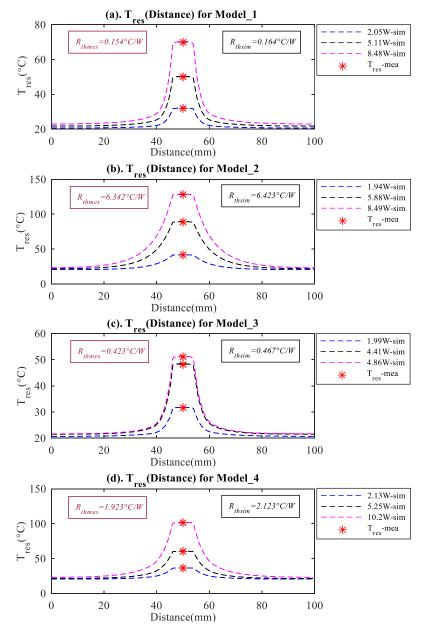
Fig.3-25. Temperature measurements of the heating source and comparisons with 3D FEM simulations
