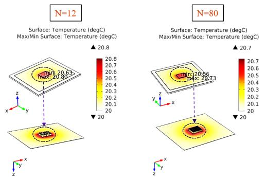
Fig.3-9. 3D FEM simulations with different number of thermal vias but the same ratios of Rol, Ro2, Ro3
