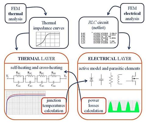
Fig.1-11. Layered approach adopted for the electro-thermal modeling of integrated power electronics modules [49]
