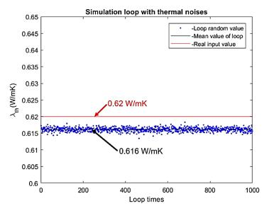
Fig.3-34. Prediction of thermal conductivity of the PCB substrate for IHCM with two unknown system parameters (Annex D)
