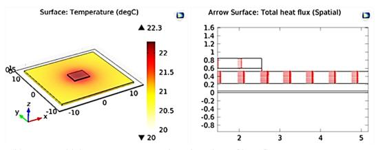
(b). Copper thickness  $e_c=300 \ \mu m$  and section view of heat flux
