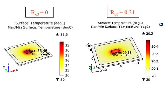
Fig.3-13. 3D FEM simulations with different ratio of via plating thickness
