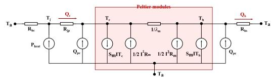
Fig.4-15. Thermal resistance network of the studied structure
