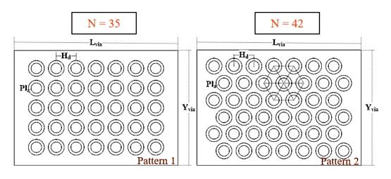
Fig.3-15. Arrangement of thermal vias in two patterns with the same available via-cluster surface
