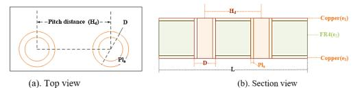
Fig.3-3. Top and Section view of the PCB substrate with two thermal vias
