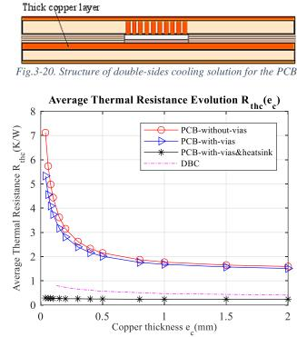
Fig.3-21. Thermal resistance evolution following the copper thickness for the same breakdown voltage 10kV
