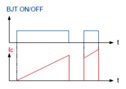
Fig.1-17. Double pulse waveform [87]
