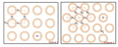
Fig.3-6. Two typical via-cluster patterns
