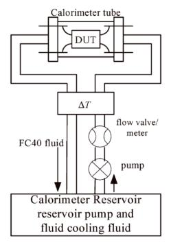
Fig.1-21. Block diagram of calorimeter [96]
