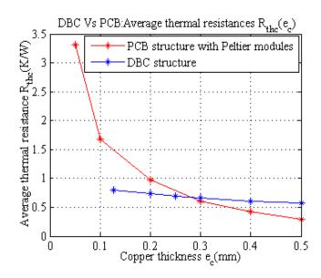
Fig.4-6. Thermal performance comparison between PCB and DBC structures. A heat dissipation of 1 W in the chip, an equivalent convection heat-transfer coefficient of 15  $W/(m^2K)$  from all external surfaces (except the bottom layer and the top TEC plate) and an ambient temperature of 25 °C are applied.
