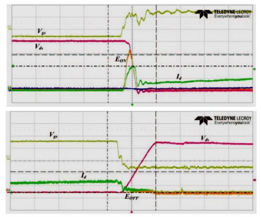
Fig.1-18. SiC MOSFET switch on and switch off transient [89]
