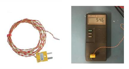
Fig.2-9. K&T type thermocouple (ANSI MC96.1) [160] and thermometer
