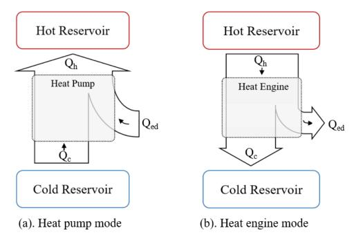
Fig.4-3. Working mode of the Peltier device
