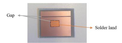
Fig.2-15. Prepared PCB substrate for chip soldering
