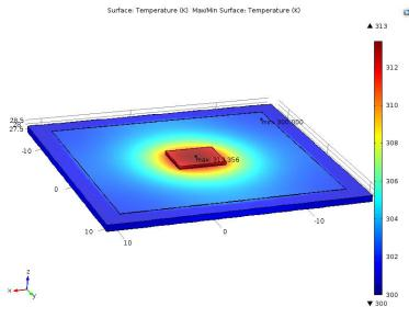
Fig.2-13. 3D Thermal simulation of the PCB structure
