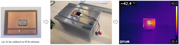
(b). Assembly fastened to radiator
