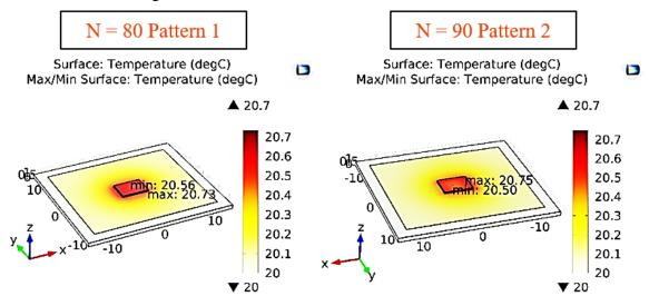
Fig.3-14. 3D FEM simulations with different via patterns
