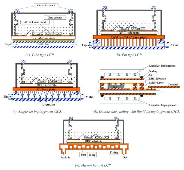
Fig.1-26. Different liquid cooling solutions [123]
