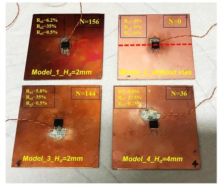
Fig.3-22. Four PCB structures with different via patterns
