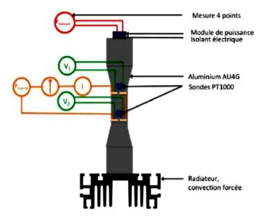
Fig.1-22. Schematic of calorimetric method with heat-flux sensors PT100 [116]
