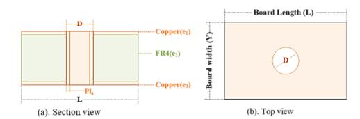
Fig.3-1. Typical PCB structure with a single thermal via
