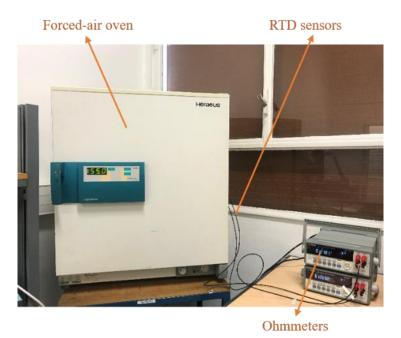
Fig.2-3. Test bench for calibrating RTD sensors
