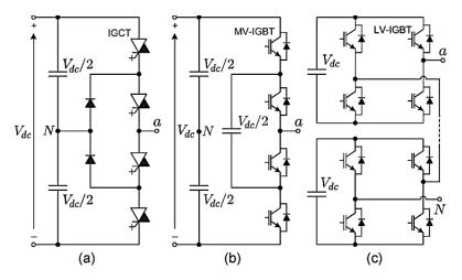
Fig.1-3. (a) Three-level NPC featuring IGCTs; (b) Three-level FC featuring MV-IGBTs; (c) Five-level CHB featuring LV-IGBTs [11]
