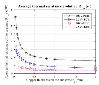
Fig.3-18. Thermal resistance evolution following the copper thickness
