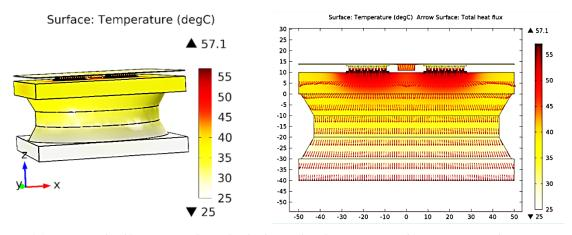
Fig.4-17. An example of 3D FEM simulation for the designed cooling structure and its section view. The PCB structure is put on a duralumin column for power loss measurement. The bottom side of the column is set at 25 °C. Heat power in the heat source  $P_{heat} = 7.6W$  and the input current in each Peltier device is 1.5 A.
