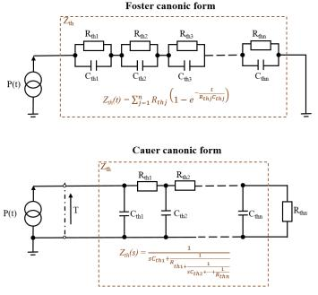
Fig.1-9. The Foster (top) and Cauer (bottom) canonic forms of thermal networks
