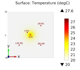
Fig.3-31. Temperature measurements on the top surface of PCB structure by 3D FEM simulations
