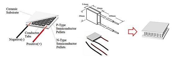
Fig.4-7. 3D model of Peltier device CP39236H
