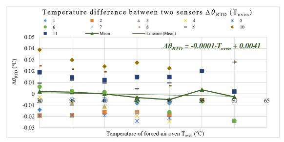
Fig.2-5. Temperature differences between two RTDs after calibration
