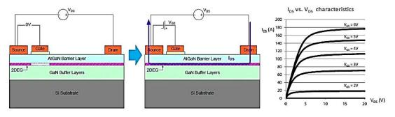
Fig.1-2. Normally-on GaN device built on a silicon substrate (Source: MOUSER ELECTRONICS [15])
