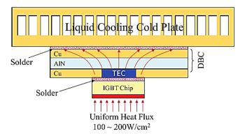
Fig.1-32. Hybrid solid- and liquid-cooling designs for IGBT isothermalization [117]
