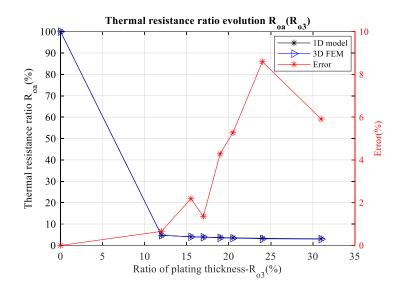
Fig.3-12. Evolution of thermal resistance ratio  $R_{oa}$  following the ratio of via plating thickness  $R_{o3}$
