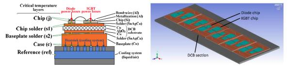
Fig.1-14. Schematic of high power IGBT module modeled in ANSYS Icepak for FEM analysis [66]
