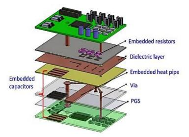
Fig.1-33. Embedded thermal solutions for PCB structures using PGS and heat pipe techniques [127]
