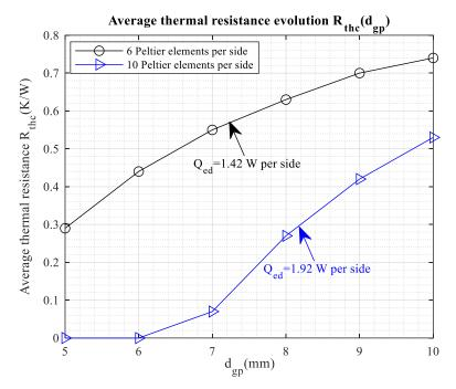
Fig.4-5. Thermal resistance evolution following the distance  $d_{sp}$ . A heat dissipation of 1 W in the chip, an equivalent convection heat-transfer coefficient of 15 W/( $m^2$ K) from all external surfaces (except the bottom layer and the top TEC plate) to the ambient and a copper thickness  $e_c$  of 500µm on the top of the PCB substrate are applied. The ambient temperature is at 25 °C.
