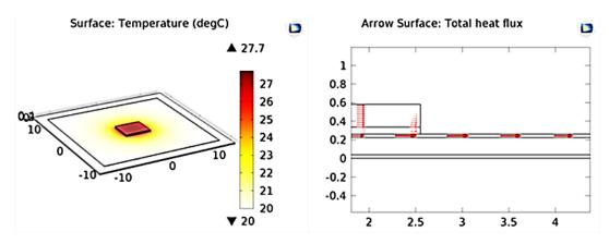
(a). Copper thickness  $e_c=38\mu m$  and section view of heat flux
