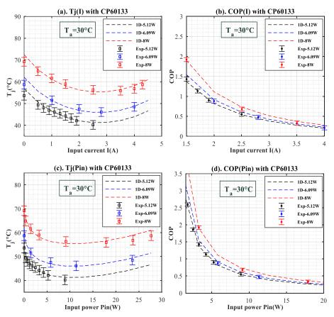
*Fig.4-25.* Experimental and estimated results with Peltier devices CP60133. (a). Junction temperature profile Tj (I); (b). Cooling efficiency profile COP (I); (c). Junction temperature profile Tj (Pin); (d) Cooling efficiency profile COP (Pin). The ambient temperature is 30 °C.
