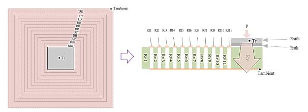
Fig.2-11. Top and section view of lumped parameter model for the PCB structure
