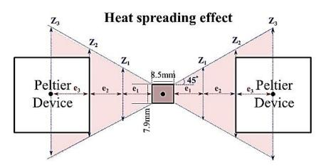
Fig.4-16. Top view for heating resistor and Peltier devices
