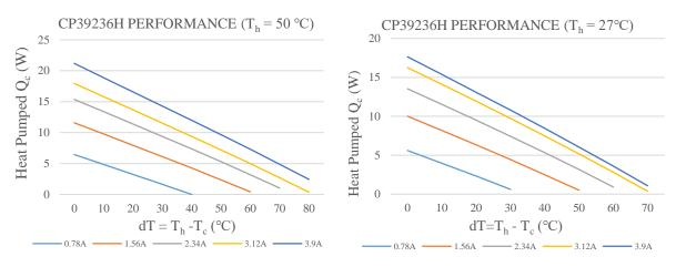
(a).  $T_h = 50 \ ^{\circ}\text{C}$  (b).  $T_h = 27 \ ^{\circ}\text{C}$ Fig.4-10. Simulation results of the heat absorbed versus temperature difference
