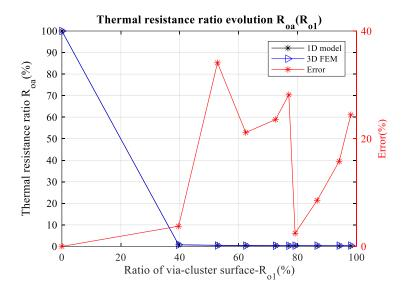
Fig.3-10. Evolution of thermal resistance ratio Roa following the ratio of via-cluster surface Rol
