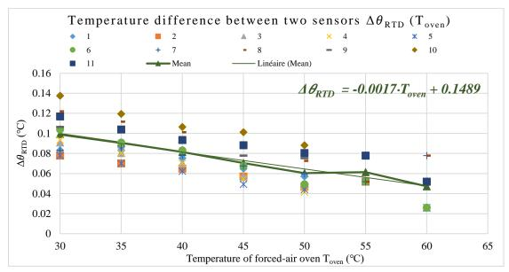
Fig.2-4. Temperature differences between two RTDs following temperature of forced-air oven
