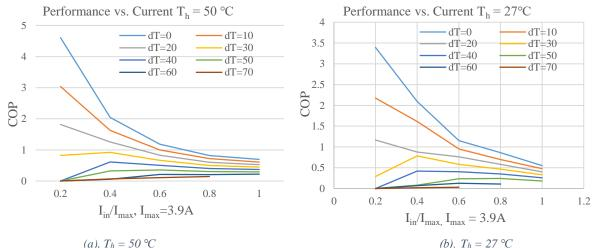
Fig.4-11. Simulation results of the relationship between COP and input current
