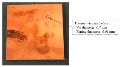
Fig.2-17. Electroplated vias in the standard PCB substrate
