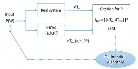
Fig.3-28. Input power estimation step for IHCM
