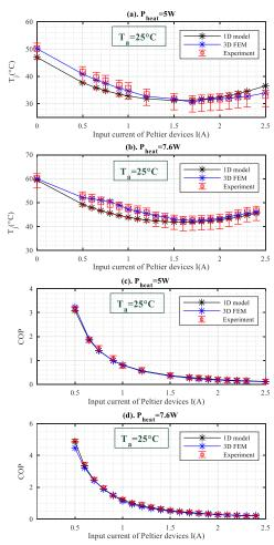
Fig.4-22. Experimental and estimated results with Peltier devices CP39236H. (a). Junction temperature profile Tj (1) when dissipating 5 W from the heating source; (b). Cooling efficiency profile COP (I) when dissipating 5 W from the heating source; (c). Junction temperature profile Tj (I) when dissipating 7.6 W from the heating source; (d) Cooling efficiency profile COP (I) when dissipating 7.6 W from the heating source. The ambient temperature is  $25 \,^{\circ}$ C.
