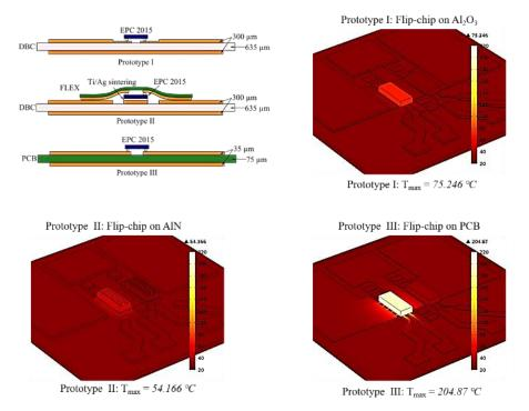
Fig.1-7. Thermal simulation results for different GaN prototypes [10]
