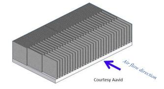
(e). Advanced heat sink with increasing fin density along air flow direction Fig.1-25. Different air cooling systems design with heat sinks [120]
