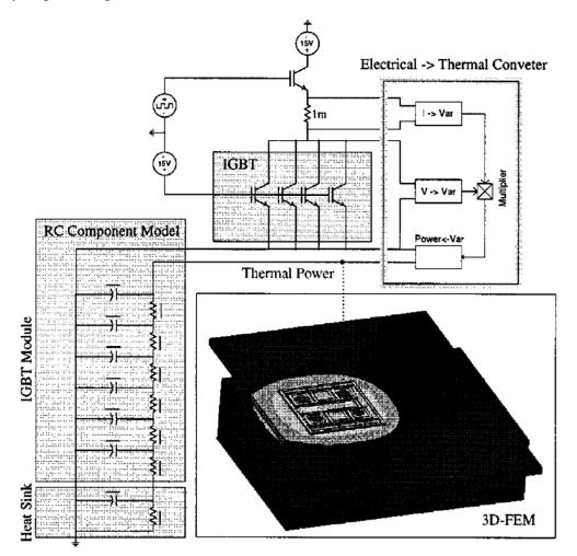
Fig.1-15. Electro-thermal model in Saber [72]
