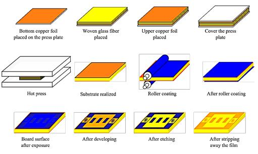
Fig.2-14. Fabrication process of PCB [161]
