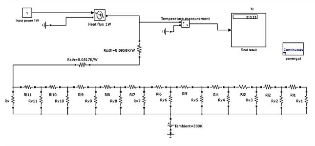
Fig.2-12. Steady-state thermal network for the PCB structure
