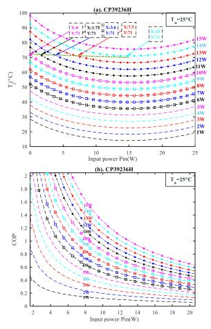
*Fig.4-24. Estimated results with Peltier device CP39236H. (a). Junction temperature profile*  $T_j$  ( $P_{in}$ ). (b). Cooling efficiency profile COP ( $P_{in}$ ). The ambient temperature is 25 °C.
