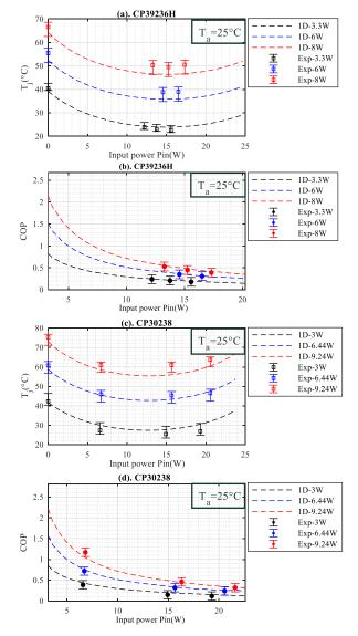
Fig.4-23. Experimental and estimated results with Peltier devices CP39236H and CP30238. (a). Junction temperature profile Tj (Pin) with CP39236H; (b). Cooling efficiency profile COP (Pin) with CP39236H; (c). Junction temperature profile Tj (Pin) with CP30238; (d) Cooling efficiency profile COP (Pin) with CP30238. The ambient temperature is 25 °C.
