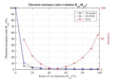
Fig.3-11. Evolution of thermal resistance ratio Roa following the ratio of via diameter Ro2
