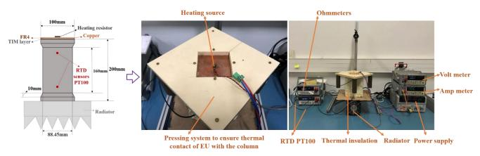
Fig.2-1. Power loss measurement test bench
