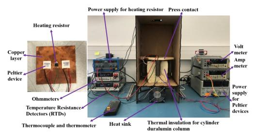
Fig.4-20. Test bench for validating the thermal models of the PCB structure with Peltier devices
