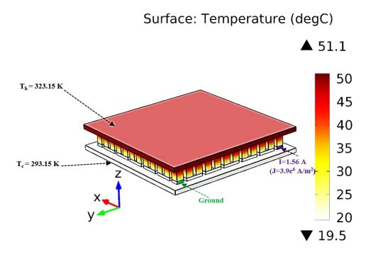
Fig.4-8. A simulated example for the 3D FEM model of product CP39236H built in COMSOL with the input current I equaling 1.56 A, the temperature of the cold side  $T_c$  equaling 20 °C, the temperature of the hot side  $T_h$  equaling 50 °C.
