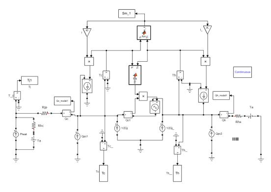
Fig.4-18. 1D electro-thermal model of the cooling structure built by Matlab Simulink
