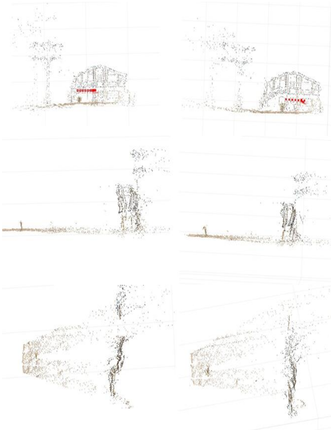
FIGURE 4.8: Reconstructed 3D scene by proposed method and GS method. 3D reconstructed scene by GS BA (left) and our proposed method (right) from front view (first row), side view (second row) and top view (third row).
