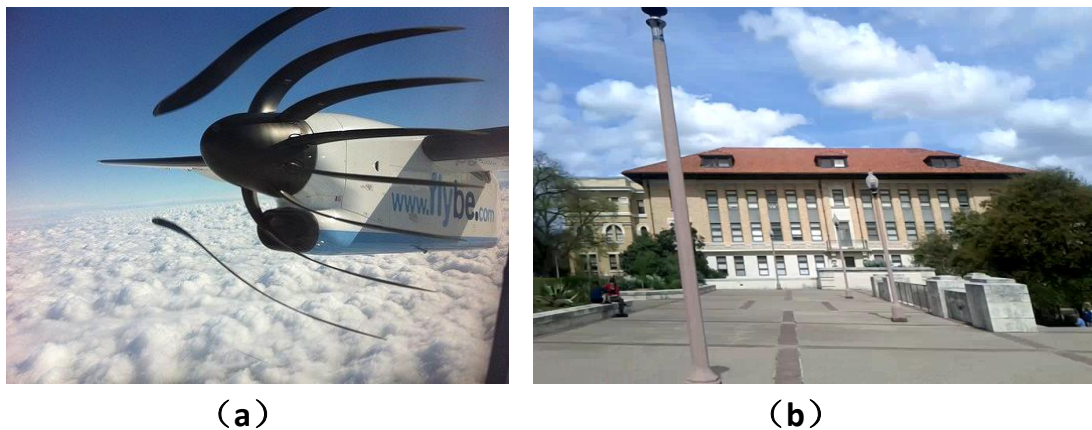
FIGURE 1.2: Images captured with a rolling shutter camera. (a) Rotating propeller captured with a static rolling shutter camera. (b) Moving rolling shutter camera, capturing a static scene. Due to the camera motion, distortion presents in the image.
