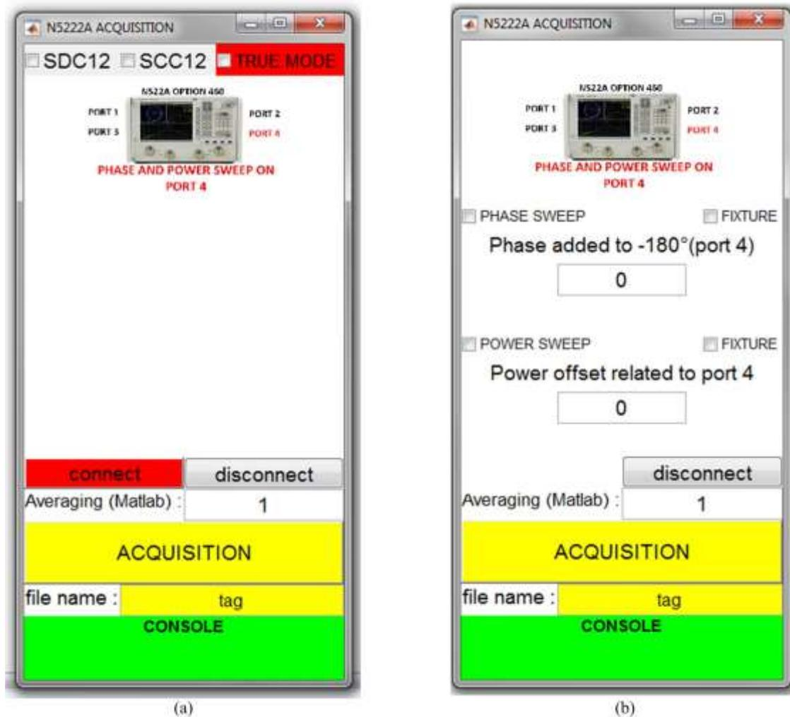
**Figure A.13.** Matlab GUI realized to acquire the Agilent N5222A VNA measuring data in balanced mode. (a) GUI that appears at software initialization before selecting the wanted measurements (Sdc12-Scs12) and before be connected with the VNA. (b) GUI after the selection of measurement and connection. It is interactive and change items visibility based on the current connection state. A console is used to inform the user about the measurement evolution.
