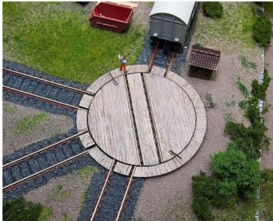
Figure 1.4: Rotating hub in railways systems
