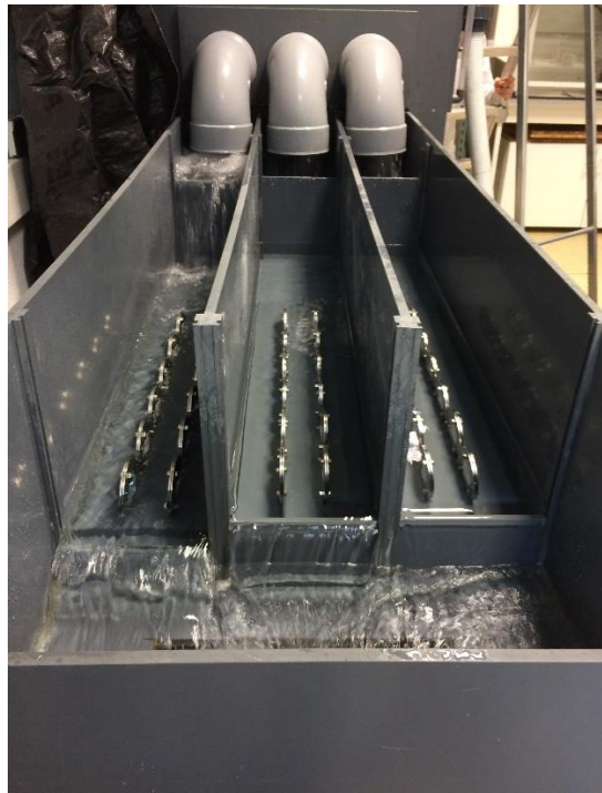
Figure V.18: View of channels during POCIS calibration.
