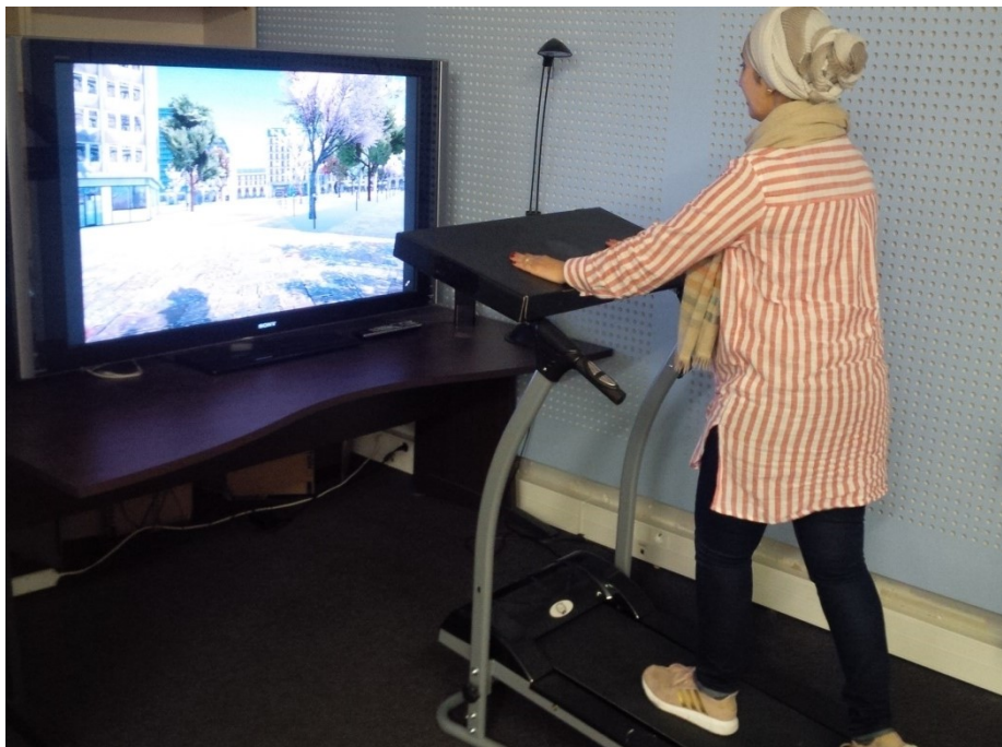
Figure 13 - experimental setup using unidirectional walking treadmill. Video learning and tasks are displayed on a large screen television
