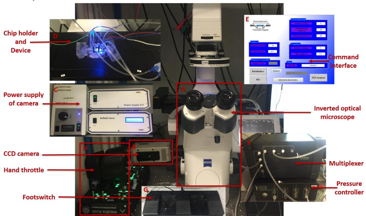
Figure 3.7: Total view photographs of the experimental bench. (A)- Inverted optical microscope. (B, C)- CCD camera and its power supply. (D)- Chip holder. (E)- Matlab® command interface. (F)- Fluid multiplexer and pressure controller. (G, H)- Footswitch and hand throttle.
