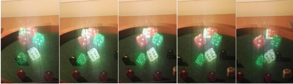
Figure 6.16: Five photographs of a rendered 3D scene taken from each viewing zone, showing transparency and the multi-view rendering. Note for example how the farther white dice is hidden behind the red dice on the right image, and visible in the left one.
