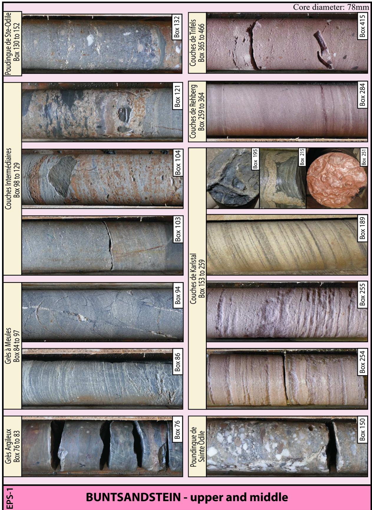
**Figure 4.6:** Photo board of the cores from the upper and middle Buntsandstein, with the Box associated with the cores; this package is correlated to a formation (with the names and boxes concerned). All the cores have a diameter of 78 mm. Box 76, Grès Argileux (upper Grès à *Voltzia*) composed of micaceous sandstone and dolomitic sandstone alternating with green to red-colored clays and silty clays. Boxes 86 and 94, Grès à Meules
