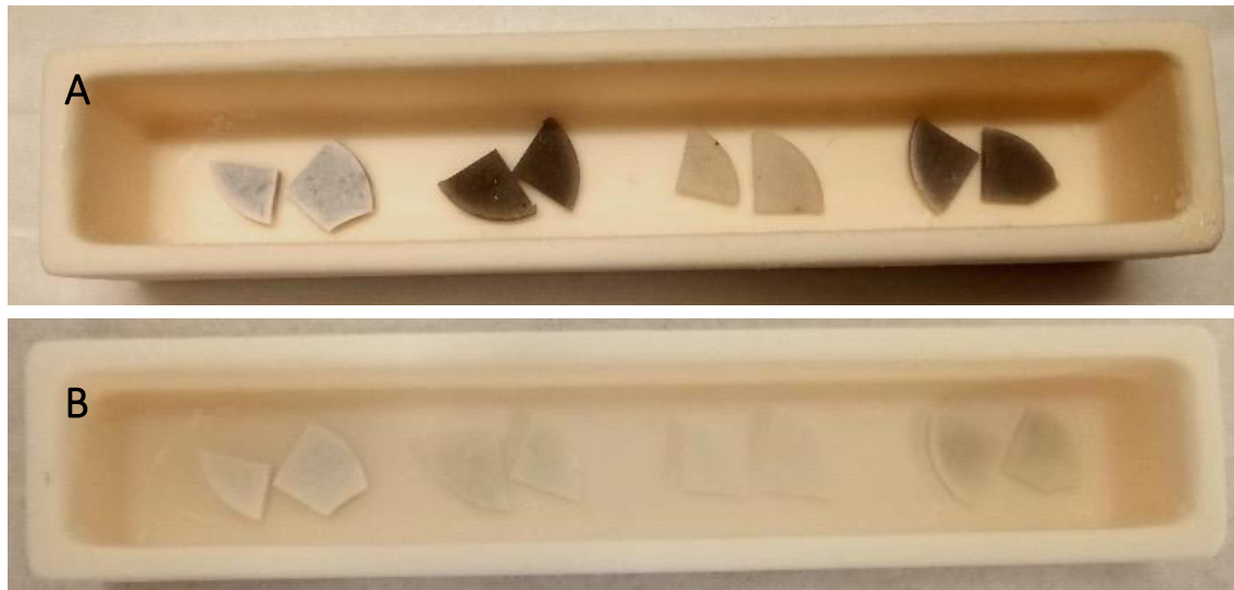
Figure 65. A: 2c, 5c, 9c and 12c samples after 30-minute 1300°C annealing in air; B: Samples after additional 4-hour annealing under oxygen flow at 1350°C.
