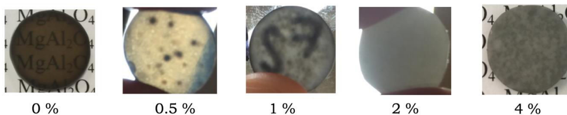
Figure 73. Optical images of spinels sintered from the commercial powder with various levels of Ta 2 O 5 doping.
