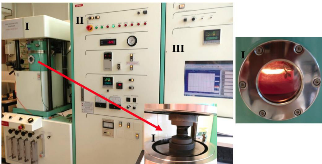
Figure 21. SPS system and sample placement, sample at high temperature.
