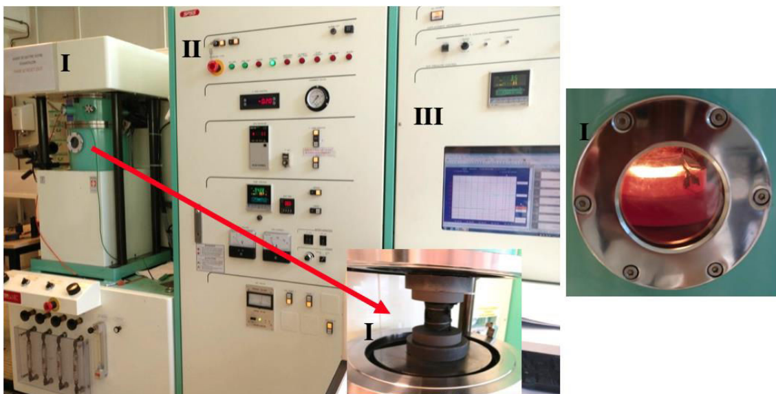
Figure 21. SPS system and sample placement, sample at high temperature.
