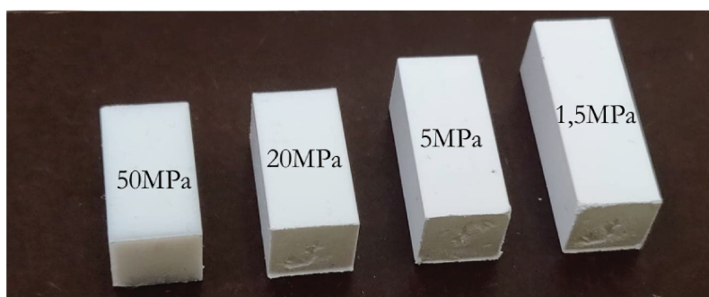
Figure 4.4: Picture of 1 g PTFE compacts for various compaction pressures (50, 20, 5 and 1.5 MPa). It appears that the light diffusion is evolving with the compaction. The difference is obvious for the 50 MPa sample.
