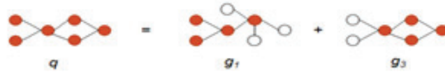
Figure 3.6: Aggregation of subgraphs from two graphs g1 and g3 responding to the query q [Le 2012]
