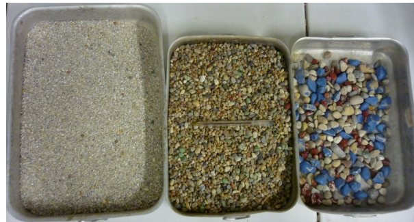
Figure 5.19 – Sieved sediment after a hooper mixture control: coarse white sand finer than 2 mm, brown and grey gravel [2;10mm] and partially painted gravel coarser than 10 mm.
