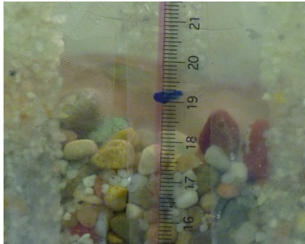
Figure 5.20 – Picture of a bed level measurement window with the transparent staff gauge. The coarse material of the bed was the biggest source of uncertainties. Here, for instance, the bed level would have been estimated as 18.1 \pm 2 \text{ mm}
