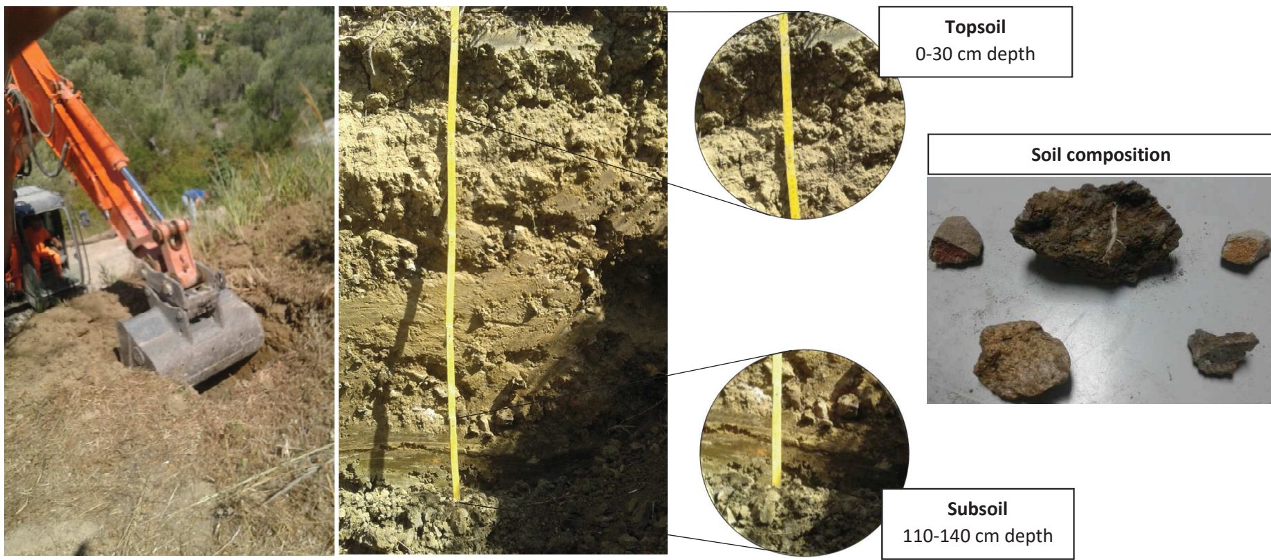
Figure 9: Excavation in Pisciotta (SA), Italy, to collect the soil for the experiment described in Chapter III and IV. Topsoil excavated from 0-30cm depth, subsoil from 110-140 cm depth. On the far right a picture with the main components of soil structure visually isolated.
