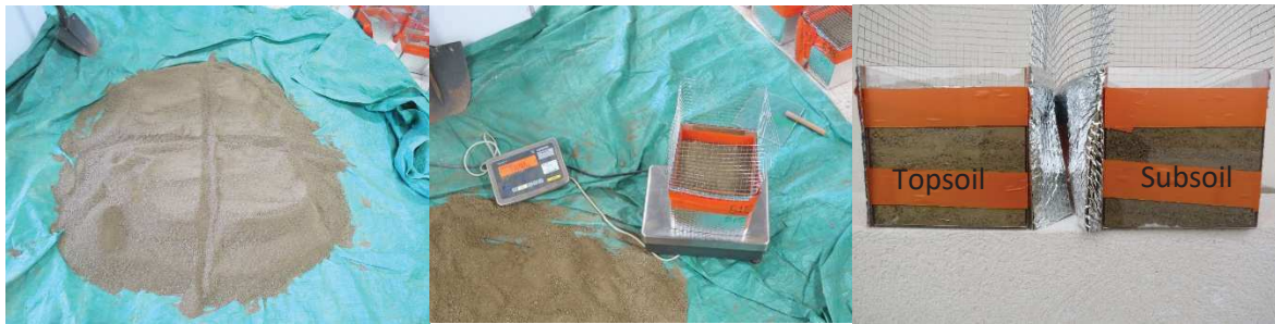
510 511 Figure S1 : Pot preparation. Starting from left to right : Quartile of soil prior to filling the pots, weighting of the pots while 512 filling and examples of two pots filled with the two different types of soil The soil has been added collecting one scoop 513 of soil from each quartile and keep moving to the next quartile, in the same order, until the desired weight was reached.
