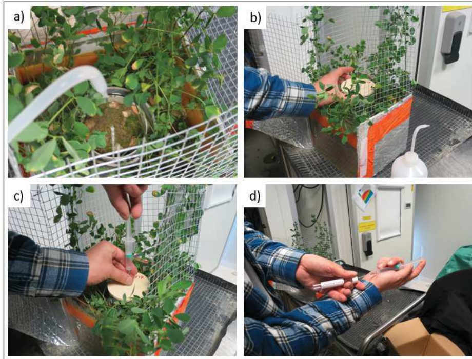
527 528 Figure S7 : Air sampling protocol : a) fill ring with water, b) place the plastic cap on top, c) take a 5ml air samples using 529 a syringe on the rubber cap and d) transfer the air taken in the airtight exainers
