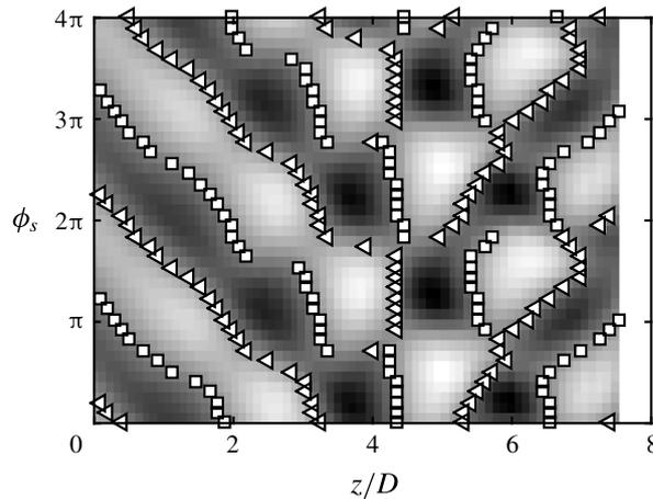
FIGURE 10. Coherent fluctuating pressure along a line at  $y = 1.5D$  against the phase with respect to screech cycle in the jet  $M_j = 1.32$  near field. The locations of the wavefronts are reported for the 40 phase steps:  $\square$ , rising edges;  $\triangleleft$ , falling edges.
