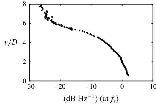
FIGURE 8. Sound pressure level (SPL) measured by the moving microphone SPL normalised by the reference microphone SPL in  $\text{dB Hz}^{-1}$  at  $f_s$ , for  $M_j = 1.35$  along the radial traverse in the nozzle exit plane.
