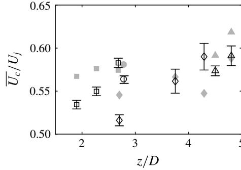
FIGURE 13. Spatially averaged convective velocity from the nozzle to the acoustic source normalised by the jet fully expanded velocity  $\bar{U}_c/U_j$ , against the acoustic source location  $z_N$ :  $\square$ , A1 mode;  $\circ$ , A2 mode;  $\diamond$ , b mode;  $\triangle$ , B mode; filled markers are from the wavenumber analysis; empty markers are from the phase analysis.
