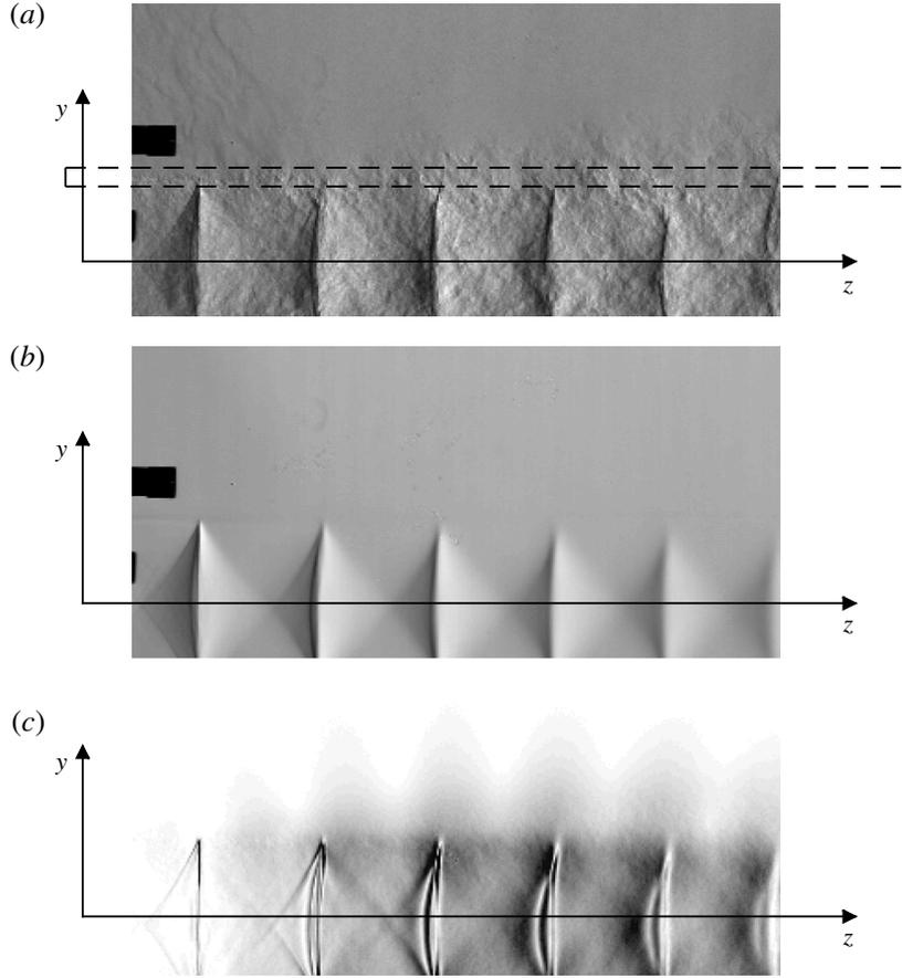
FIGURE 4. (a) Instantaneous schlieren image  $g(y, z, t)$  ( $4 \mu\text{s}$  time exposure). The dashed rectangle shows the field of view of the high-speed records. (b) Averaged field  $\bar{g}(y, z)$ . (c) Fluctuating field  $G_s(y, z)$  at the fundamental screech frequency from schlieren measurement of a jet at  $M_j = 1.15$ , mode A2.
