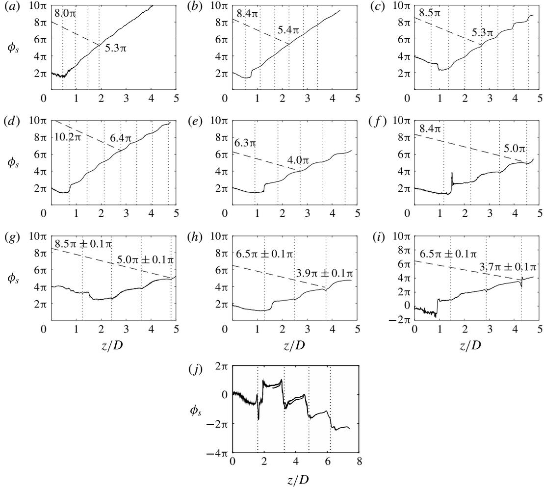
FIGURE 12. Phase evolution  $\phi_s = 2\pi t/T_s$  extracted from the cross-spectrum between a pixel at the nozzle and a pixel moving along the line  $y/D=0.55$ : ---, acoustic feedback at  $337 \text{ m s}^{-1}$ ; shock locations are indicated by vertical dotted lines. Jet Mach number: (a)  $M_j = 1.07$ , (b)  $M_j = 1.10$ , (c)  $M_j = 1.13$ , (d)  $M_j = 1.15$ , (e)  $M_j = 1.23$ , (f)  $M_j = 1.32$ , (g)  $M_j = 1.35$ , (h)  $M_j = 1.37$ , (i)  $M_j = 1.45$  and (j)  $M_j = 1.50$ .
