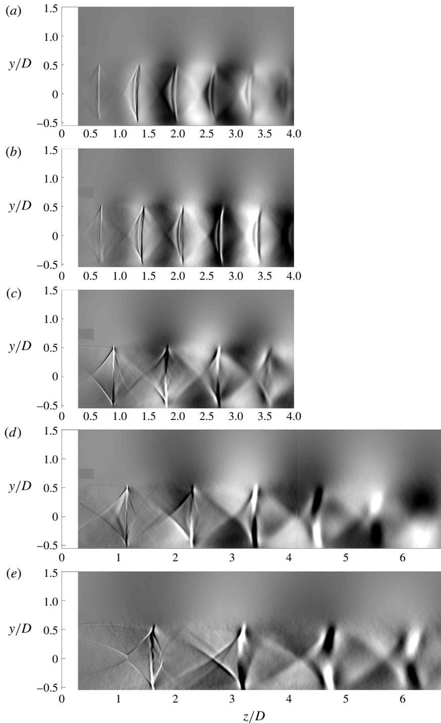
FIGURE 14. Real part of the Fourier transform at the screech frequency calculated from schlieren films: (a)  $M_j = 1.13$  mode A1, (b)  $M_j = 1.15$  mode A2, (c)  $M_j = 1.23$  mode b, (d)  $M_j = 1.32$  mode B, (e)  $M_j = 1.50$  mode b. Results from two schlieren records are juxtaposed in (d) and (e).
