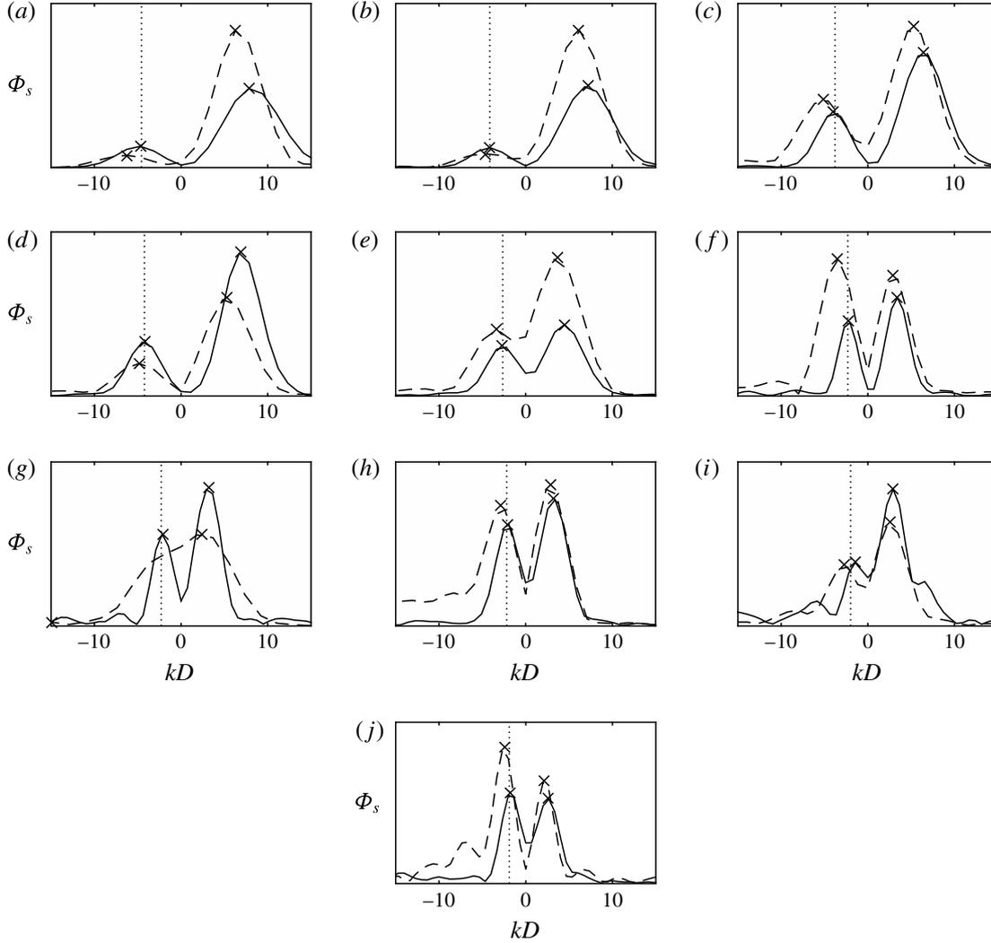
FIGURE 6. Wavenumber spectrum at screech frequency  $\Phi_s$  (arbitrary linear scale) upstream of the source (—) and downstream (---): (a)  $M_j = 1.07$ , (b)  $M_j = 1.10$ , (c)  $M_j = 1.13$ , (d)  $M_j = 1.15$ , (e)  $M_j = 1.23$ , (f)  $M_j = 1.32$ , (g)  $M_j = 1.35$ , (h)  $M_j = 1.37$ , (i)  $M_j = 1.45$  and (j)  $M_j = 1.50$ . The wavenumber  $k_s = -\omega_s/c_0$  is indicated by the vertical dotted line.
