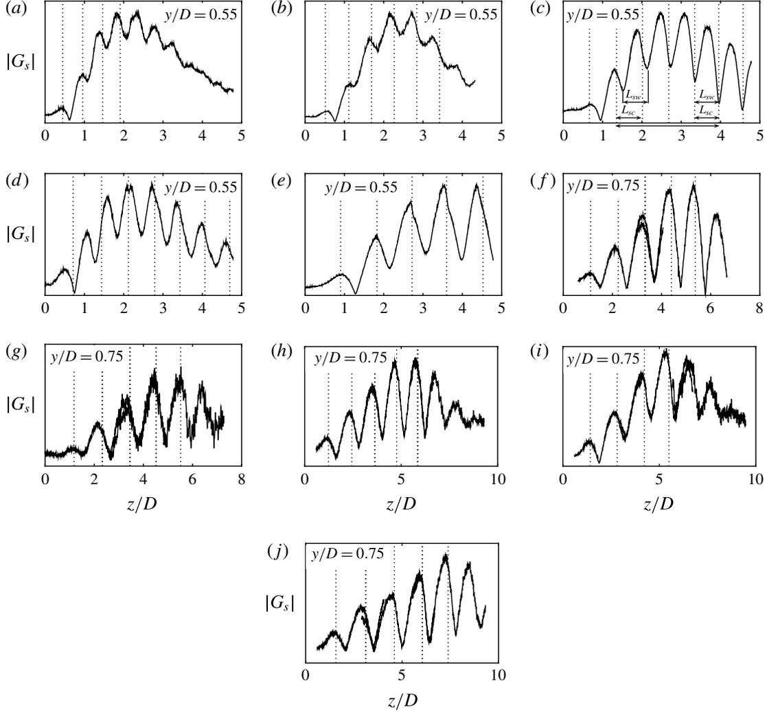
FIGURE 5. Modulation of the grey-level field  $G_s$  at the screech frequency (arbitrary scale) along a line at  $y/D = 0.55$ : (a)  $M_j = 1.07$ , (b)  $M_j = 1.10$ , (c)  $M_j = 1.13$ , (d)  $M_j = 1.15$ , (e)  $M_j = 1.23$ , (f)  $M_j = 1.32$ , (g)  $M_j = 1.35$ , (h)  $M_j = 1.37$ , (i)  $M_j = 1.45$  and (j)  $M_j = 1.50$ . Shock locations are indicated by vertical dotted lines.
