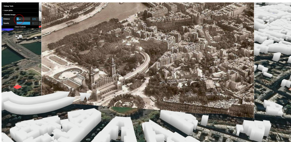
(b) Pose estimation of a historical aerial image of Trocadero square (Paris, France) that was registered (Harrach et al., 2019) to a city 3D model visualized with iTowns 4 (Devaux et al., 2012).
