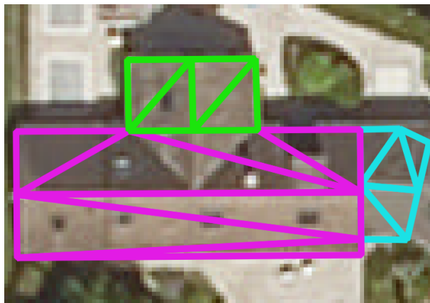
Figure 3.4: Nadir projection of an erroneous building superposed on the corresponding orthoimage showing a BOS error. We can see how a single building that was modeled into three different ones depicted here in three different colors.
