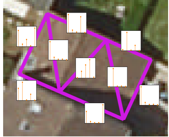
(b) Histograms describing the similarity between edges and the orthoimage.
