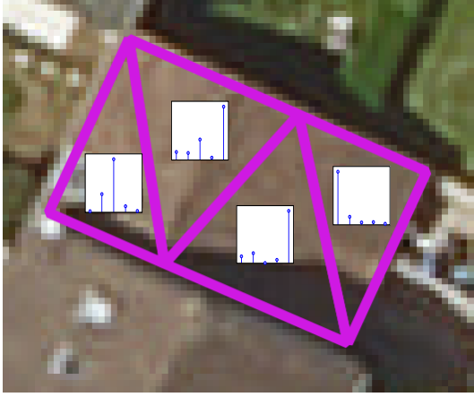
(a) Depiction of histograms describing the similarity of each of the model’s projected facet to the orthoimage.
