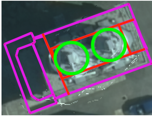
Figure 3.17: Nadir projection of an erroneous building superposed on the corresponding orthoimage showing a FIT error. The true form (in green) of the towers that is completely misrepresented (in red).
