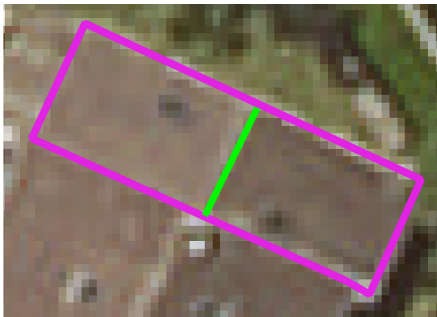
Figure 3.11: Nadir projection of an erroneous building superposed on the corresponding orthoimage showing a FUS error. It shows a case where a higher neighboring building part can drive a misestimation of both facet planes which end up confused in one flat roof. The line segment highlighted in green gives away the fact that the roof was undersegmented.
