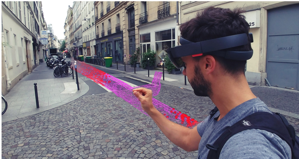
(a) Virtual visualization of sewers in Paris based on the 3D model of the city (Devaux et al., 2018).
