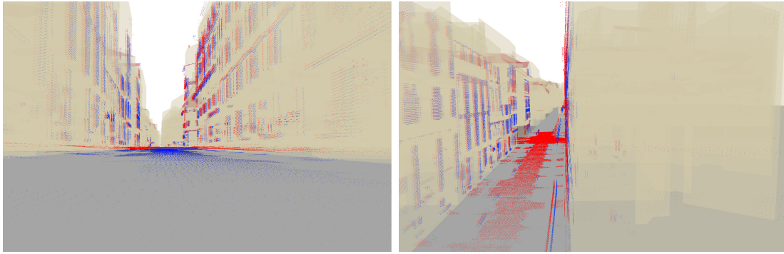
Figure 1.14: Terrestrial LiDAR point clouds are registered against 3D building models. The registered point clouds can be used to enrich the 3D models with detailed reconstructions of façades. The raw point cloud is represented in red while the registered one is illustrated in blue. Image taken from (Monnier, 2014).
