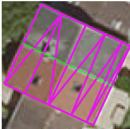
Figure 3.3: Nadir projection of an erroneous building superposed on the corresponding orthoimage showing a BUS error. We can recognize, based on the color differences of roof tiles, the existence of two buildings instead of one.
