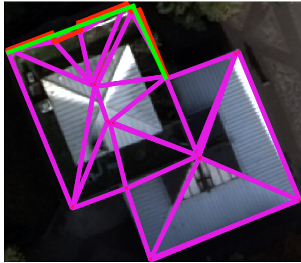
Figure 3.8: Nadir projection of an erroneous building superposed on the corresponding orthoimage showing a BIT error. We can identify (in green) the correct footprint shape compared to the one that was reconstructed (in red).
