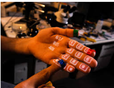
Figure 3.17: Sixth sense detects touch on skin with a 2D camera
