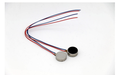
Figure 3.2: Vibration motors present in most smartphones.
