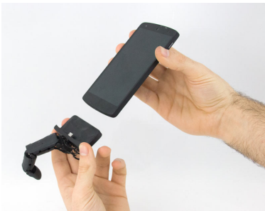
Figure 6.11: MobiLimb is plug and play and can easily be connected to most of existing device.
