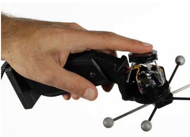
Figure 3.9: NormalTouch stimulates fingertip with small-size distributed touch-screen capable to create textures.
