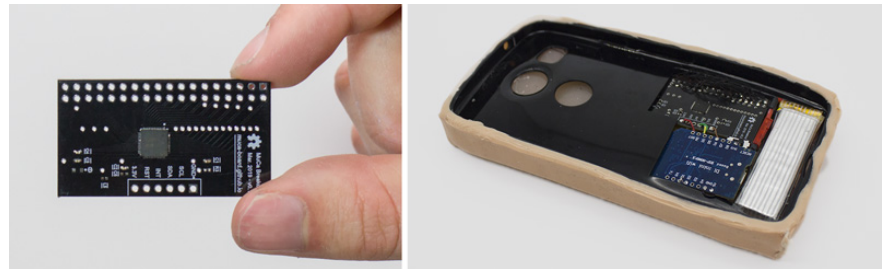
Figure 8.9: Left. Open Hardware Mutual Capacitance breakout Right. Smartphone case prototype hardware.
