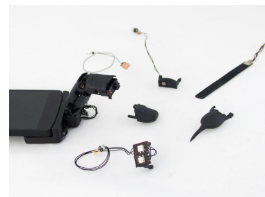
Figure 6.12: MobiLimb supports several modular tips (e.g. LED, shells, proximity sensors) to create new forms of interaction.
