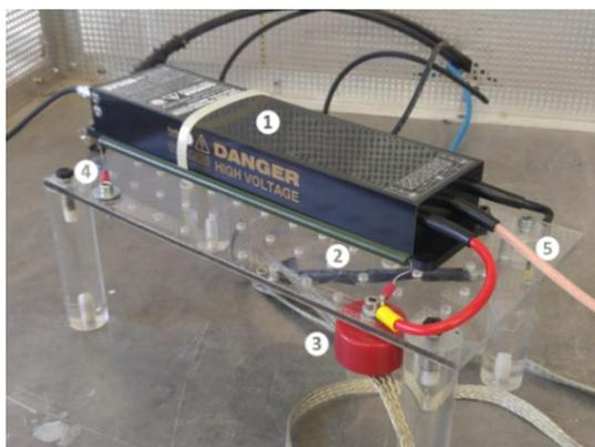
**Figure 30: Behlke solid state HV switch applied in PLI process for nanoparticle synthesis. It is composed by:**
