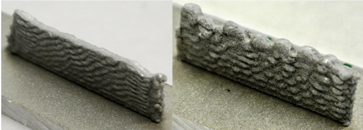
Figure 5.87: Single-track wall deposit by LMD of allow powder 224.0-A 80-100 \mu m using parameters from trial 8 (left) and trial 5 (right)
