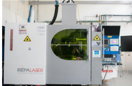
Figure 1.14: MultiCLAD LF4000 LMD system at the Rapid Manufacturing Platform of Ecole Centrale de Nantes
