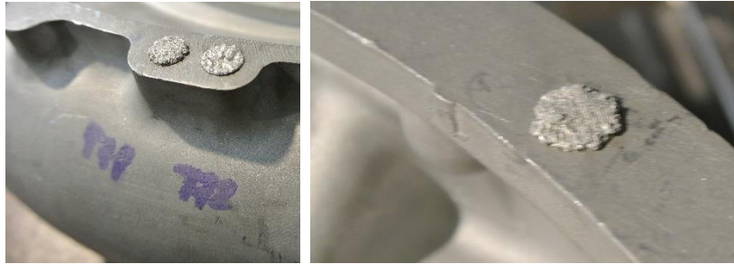
Figure 5.98: Examples of repaired cavity samples on a premium high-strength Al-Cu
