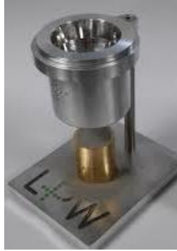
Figure 2.22: Standard Hall Flowmeter testing
