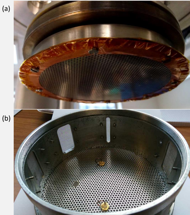
Figure SII.2-3: Pictures of the resonant cavity. (a) Top part, with a copper crown and its insulating tape. (b) Lower part, in the case of 2 loop antennas.
