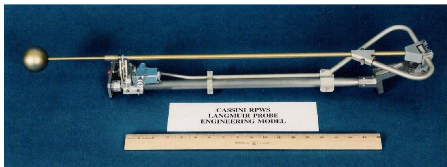
Figure IV.1-3: Engineering model of the Cassini RPWS Langmuir Probe, folded. © Swedish Institute of Space Physics.
